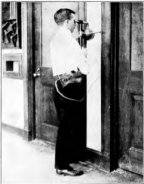
FIG. 2.—Method of using instrument to measure the reflection factor of a wall
